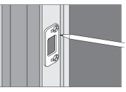
4c If necessary, use chisel, hammer and drill to correct door jamb preparation.
